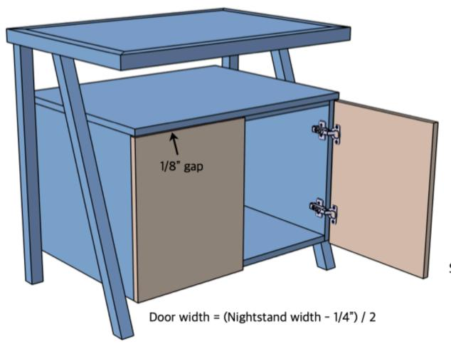
Cut doors to final dimensions and edge band perimeters.
