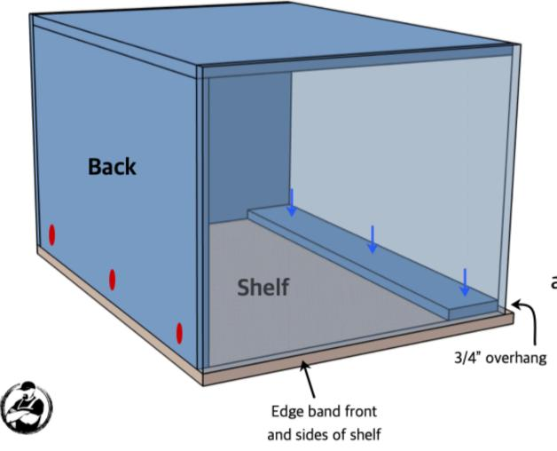
Edge band front and sides of the shelf and install using 1-1/4" pocket screws and 1-1/4" wood screws.
