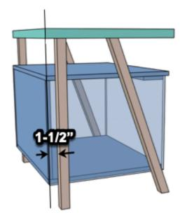
Mark the 2x2 locations, remove and drill a pilot hole through cabinet. Then, relocate 2x2s and secure with wood glue and 2" wood screws. Pre-drill top and attach with 3" wood screws. Sink screw heads below surface and fill with wood filler.
